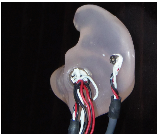
Figure 1: Assembled earpiece, from [6]. 3 microphones and 2 receivers are fitted into an individual silicone earmould.
