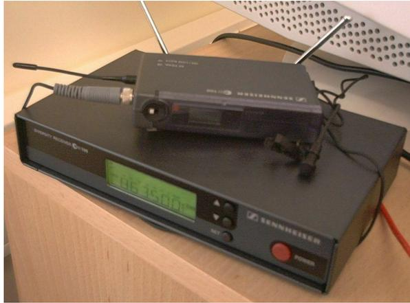
Figure 6: Sennheiser EW112 wireless receiver and transmitter (incl. microphone)
