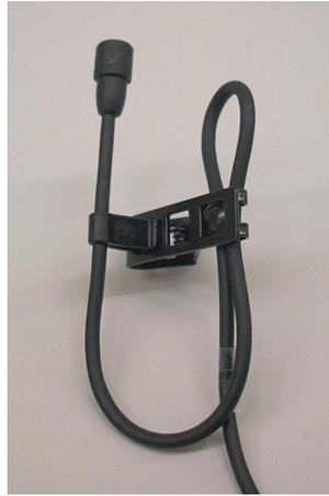
Figure 2: Sennheiser MKE 2-5-C (with tie-clip)
