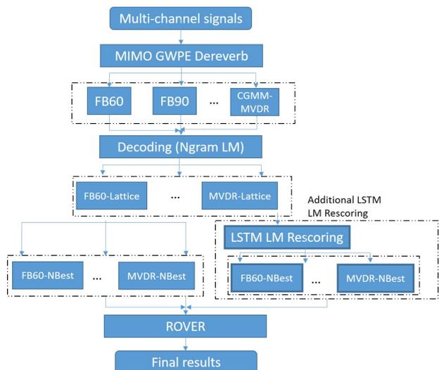
Figure 1: Flowchart of ROVER over multiple beamformed outputs.
