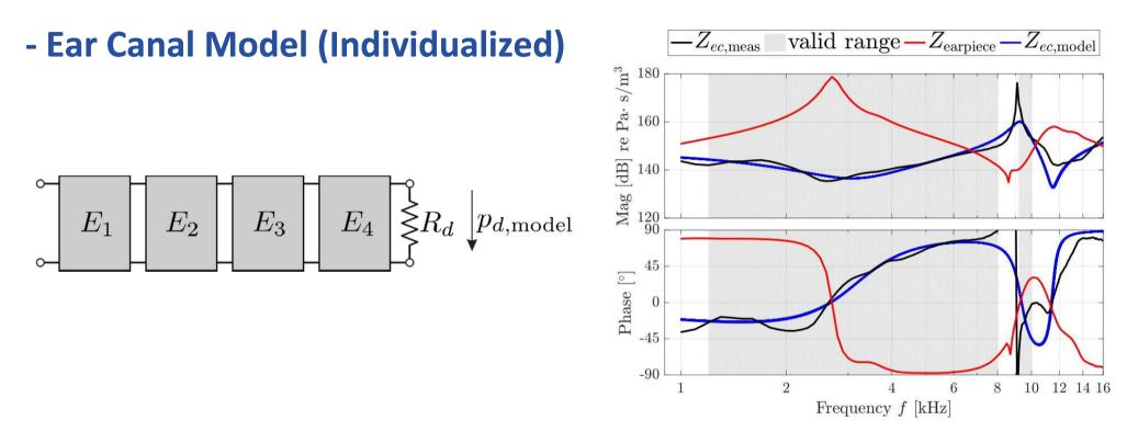
**Parameter optimization** (4 radii, 1 length, 1 resistive load) by minimizing the difference between measured and modeled ear canal (Nelder-Mead simplex optimization procedure):
