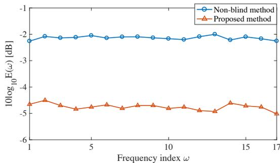
Figure 5: Experimental results obtained when the reverberation time  $T_r$  was 1.5 s. The vertical axis represents  $E(\omega)$  of the logarithmic scale and the horizontal axis represents the frequency index  $\omega$  in FWF.
