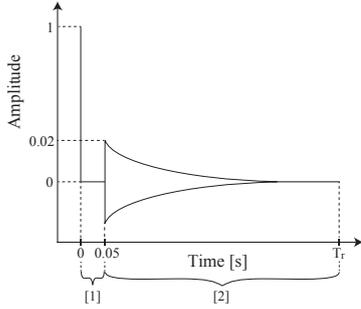
Figure 2: Pattern diagram of the room impulse response based on the model proposed by Polack [20]. The first part  $h_d(t)$  represents a direct sound and the second part  $h_r(t)$  represents a reverberation component. The border between the direct sound and the reverberation component was 50 ms.
