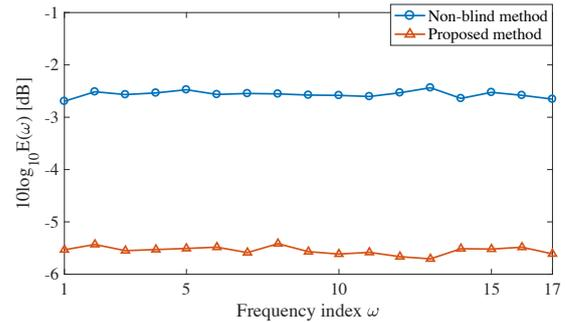
Figure 6: Experimental results obtained when the reverberation time  $T_r$  was 2.0 s. The vertical axis represents  $E(\omega)$  of the logarithmic scale and the horizontal axis represents the frequency index  $\omega$  in FWF.
