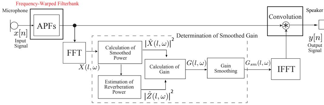
Figure 1: System overview. The input signal flows through all-pass filters (APFs) with the warping parameter to analyze the input signal. The gain function  $G(l, \omega)$  is determined by the estimated reverberation power.
