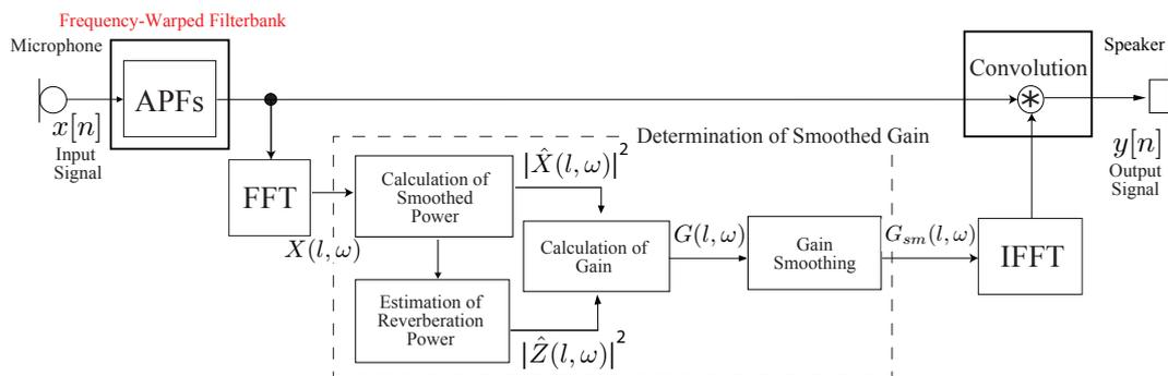
Figure 1: System overview. The input signal flows through all-pass filters (APFs) with the warping parameter to analyze the input signal. The gain function  $G(l, \omega)$  is determined by the estimated reverberation power.
