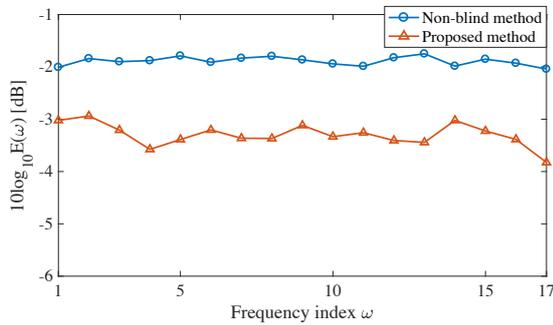
Figure 4: Experimental results obtained when the reverberation time  $T_r$  was 1.0 s. The vertical axis represents  $E(\omega)$  of the logarithmic scale and the horizontal axis represents the frequency index  $\omega$  in FWF.
